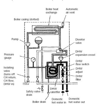
With no call for CH, the boiler fires only when DHW is drawn off. When there is a call for CH, the heating system is supplied at the selected temperature until DHW is drawn off. For the boiler shown in Figure 1, the full output from the boiler is then directed via the diverter valve to the calorifier, to supply a maximum DHW draw off (e.g. hot water taking priority over central heating).
