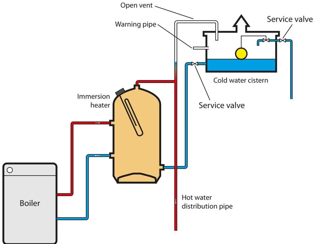
Image 2 The direct vented hot water storage system
