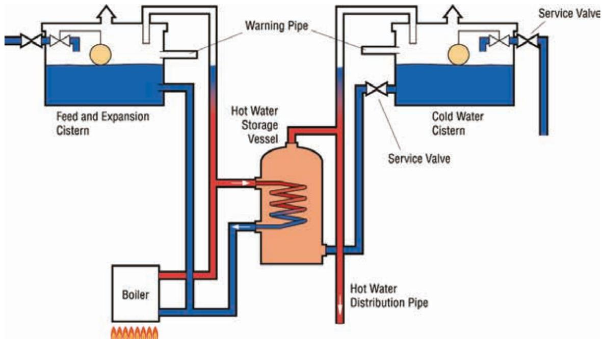
Image 3 The indirect vented hot water storage system
