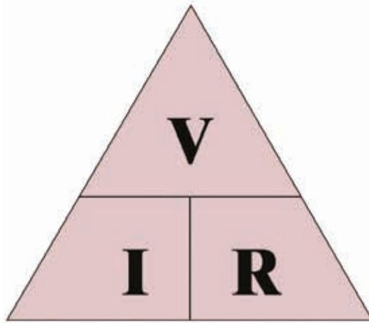
By using the Ohm's Law Triangle it is possible to calculate the quantities that make up electrical circuits in the following ways:
