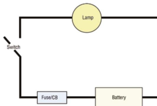
**Note:** A switch opens the circuit and **prevents** the electricity from flowing until we close it again. This is different when we think of gas and water as when we open a valve or tap we **enable** the gas or water to flow:
