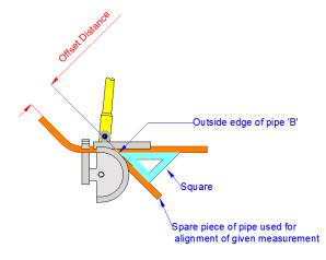
Place the pipe in the machine and if it has been set out correctly, the pipe will sit in the bending machine as shown. It can be checked for accuracy by ensuring the two legs of the bend are in line, as shown by the blue line, to give the correct offset distance.
