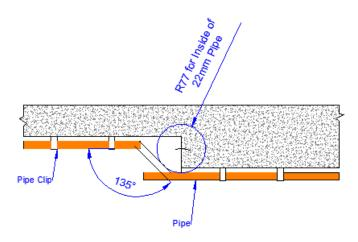
Use the drawing as a template, and decide on a fixed point, which can be a pipe clip, a fitting or something else. The pipe should be marked for bending on the outside of the first bend as shown:
