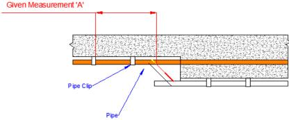
Place the pipe in the bender and using the square and a piece scrap of pipe, line up the mark as shown - Remember to keep the fixed point behind the machine.
