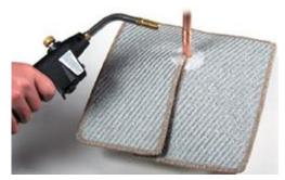
Heat proof mat – This is used to protect the fabric of the building from damage by the flame when soldering. Care should be taken when using soldering equipment and the flame should be directed away from combustible materials. Mats should only be seen as an aid. DO NOT point the flame directly at the mat. Whilst they are called heat proof mats, in fact, they are heat resistant.
