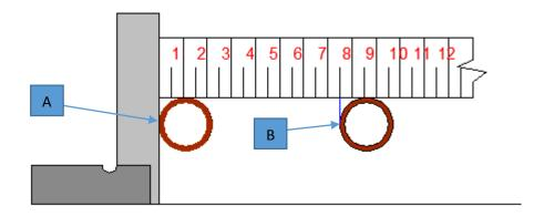
Another example is working from either a pipe end or a fixed point to the centre of a pipe.
