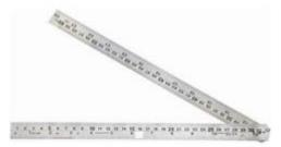
Engineers split rulers are good for checking angles when bending pipe; they can be set to the required angle and held adjacent to the pipe in the bender, to ensure bending is accurate.
