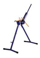
Upright stand benders are available and tend to be used for larger diameter pipes as they will bend up to 42mm pipe.
