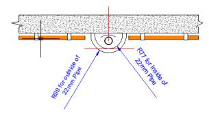
Striking through the two arcs – one at **52.5mm** and **67.5mm if using 15mm** pipe, or **77mm and 99mm for 22mm** pipe as shown.
