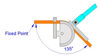
Pull the bend to the required angle and using a split rule set at the angle, or an angle finder, check that the bend is accurate before removing from the bending machine. Remember to allow for the 'spring back' when releasing the pressure on the arm.
