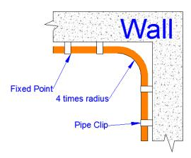
The pipe should fit in the clips without straining.
