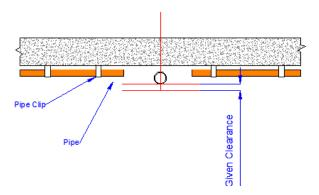
This can be achieved by drawing the passover out. In this diagram, the object to be passed over and the clearance can be seen - This is the start of our setting out.
