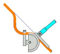
When checking, use a long steel rule to ensure that the passover is in line.
