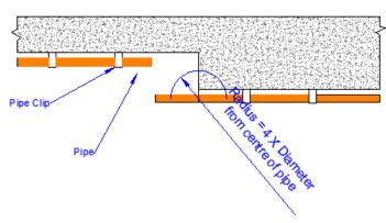
To set out, start as above then strike an arc from the centre of the pipe at 4 times the diameter as the radius, as shown:
