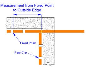
When copper pipe is to be bent, it is normal practice that all the marking out for the marking of the bending is done to the **outside edge.**
