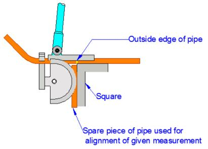
Return the pipe to the bending machine with the use of a square and a scrap piece of pipe, as shown. Remember the fixed point still needs to be inserted behind the bending machine.
