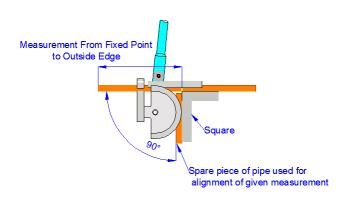
Place the pipe to the bender, ensuring the fixed point is behind the back stop. Use a scrap piece pipe and a square to ensure the mark on the pipe is aligned with the outside edge of the scrap pipe. Pull the bend to the correct angle.
