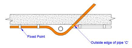
The pipe should now fit the drawing without any tweaking, as shown.
