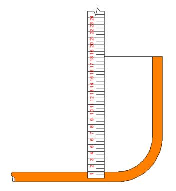
In this example you can see that guessing the distance from the centre of the Horizontal pipe to the end of the vertical pipe or fixed point is around 182mm to 183mm.
