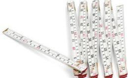
An alternative is to use a tape measure. The disadvantage of using a tape measure is that the end hook can become loose, reducing accuracy. When working to precise dimensions - plus or minus 2mm (± 2mm) - the use of a ruler is preferable.
