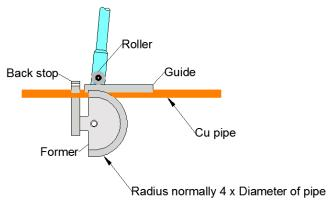
For 15mm pipe it will be 15mm x 4 = 60mm radius to centre line.
