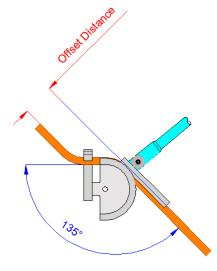
To check that the offset is in-line and parallel use a long steel rule. Then return to the drawing and it should match 100%. Check that the clearance is correct – The accepted industry tolerance is  $^+$ /- 2mm.
