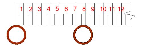
Using the above method is inaccurate because it relies on the user guessing the centres of the pipes - The measurement appears to be between 77mm and 79mm.
