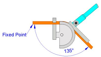
Pull the bend to the required angle. Using a split rule set at the angle (or an angle finder), check that your bend is accurate before removing from the bending machine. Remember to allow for the spring back when releasing the pressure on the arm.
